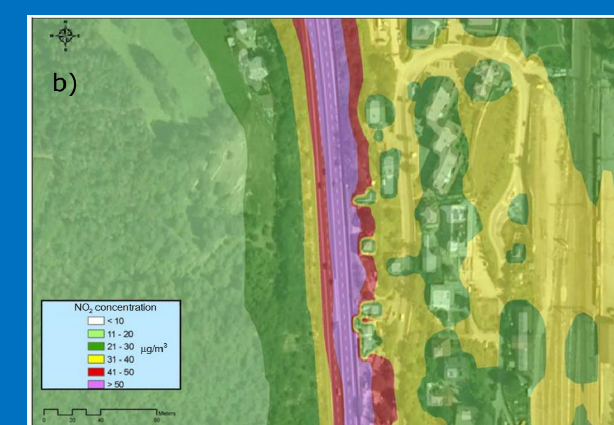
Examples of maps obtained from the WRF and the CALPUFF models. a) Forecast of wind speed at 10 m AGL in the study area; b) NO 2 concentrations along the Brenner highway.
